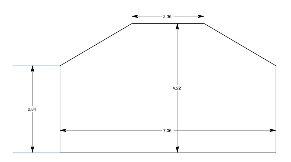
NORTH WARNBOROUGH VILLAGE HALL - MAIN HALL DIMENSIONS TO UNDERSIDE OF ROOF TRUSSES in metres, approximate Metres to feet multiplier 3.279. RB November 2014
